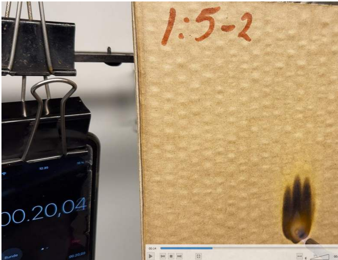
Photo 6 Testing of plate "1:5-2"
