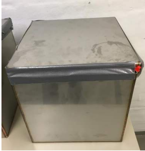
Picture 1: Stainless steel box sealed with gaffer tape and equipped with a sorbent tube
